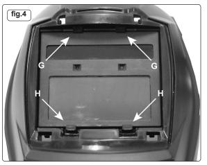
clips (see 'B' in fig.3) by pressing them downwards and forwards. Lift off the front cover. Referring to fig.4, push downwards on the two clips 'H' whilst pushing the bottom edge of the cartridge outwards from inside the 5.1.4. helmet. When it is free from the lower clips pull the cartridge downwards and forwards to free it from the upper retainers. (See 'G' in fig.4.)
